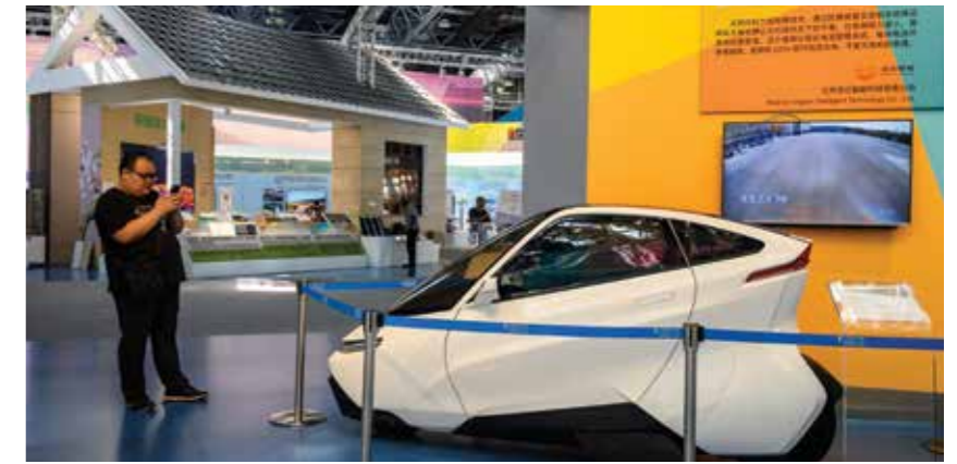
Self-balancing two-wheeled electric vehicle on display at the Exhibition Center of Zhong-guancun National Independent Innovation Demonstration Zone (Photo by Hariandi Hafid from Indonesia) 中关村国家自主创新示范区展示中心展出的自平衡两轮电动汽车。 摄影：哈里安迪·哈非德（印度尼西亚）
